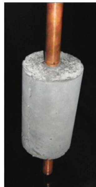
Figure 3.2 : Earth enhancement material before & after setting
