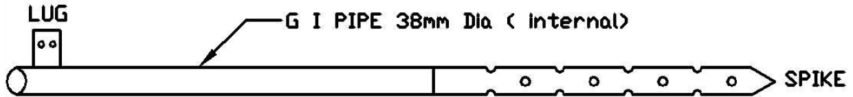
Fig.2.2: Earth electrode (GI pipe)
