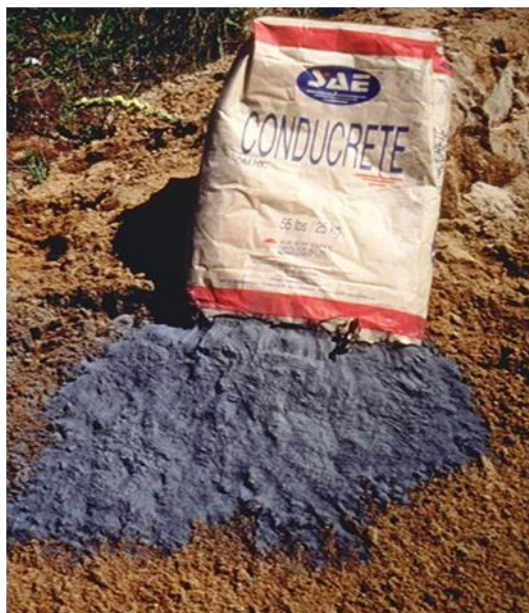
Figure 3.2 : Earth enhancement material before & after setting
